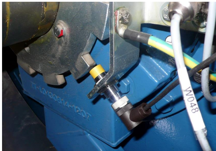
Picture 25: Radial installation of a speed sensor
